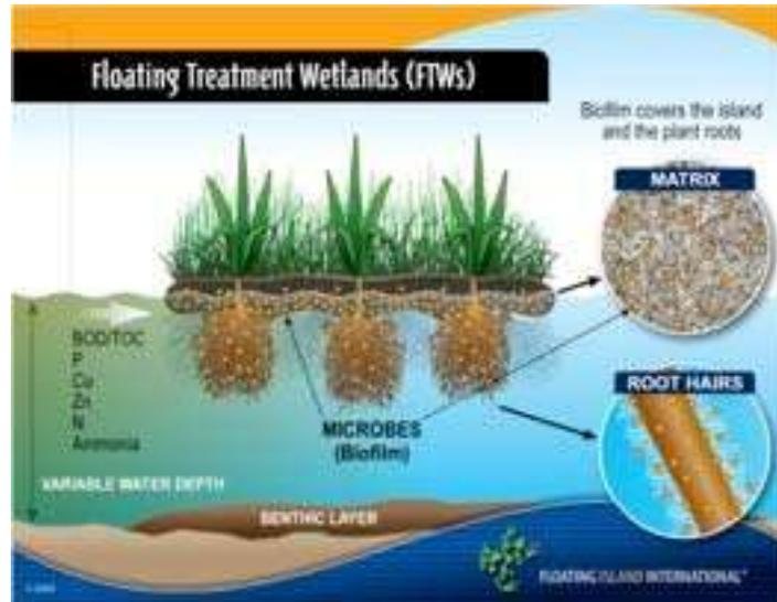
*Schematic illustration of BioHavens and biofilm*
